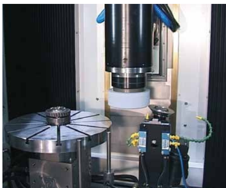
CNC dressing with rotary diamond disk
