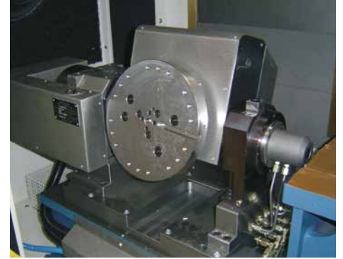
Double CNC indexing table for 5-axis continuous path controlled profile grinding
