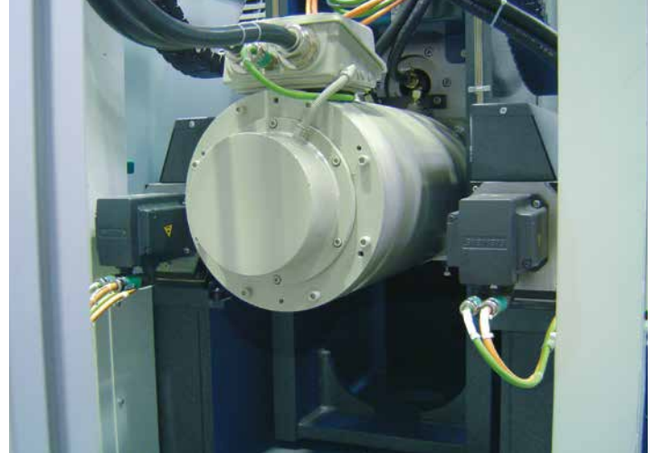
Z-axis with parallel drive system for increased rigidity (optional)
