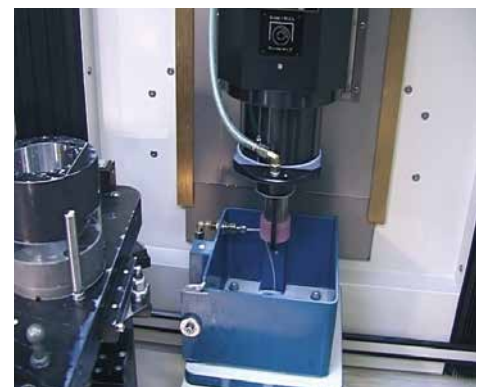
CNC dressing with single point diamond
