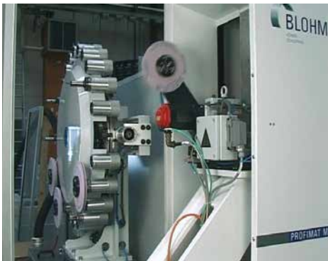
Tool changing systems with up to 24 tools 12 x D=300 or 8 x D=400
