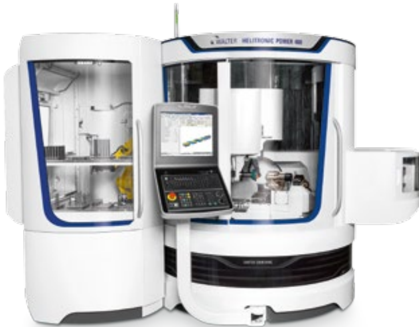
The WALTER HELITRONIC POWER 400 with wheel changer and "Robot Loader" option
