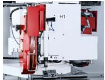
Wheelhead on the S22 for high speed grinding
