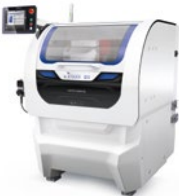
The S11 is STUDER's smallest production cylindrical grinding machine
