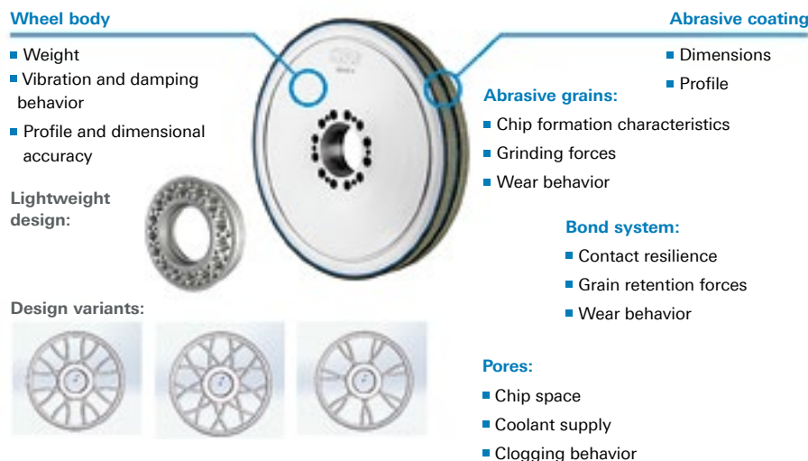
Figure 1: Design of high-performance grinding tools and wheel body variants
