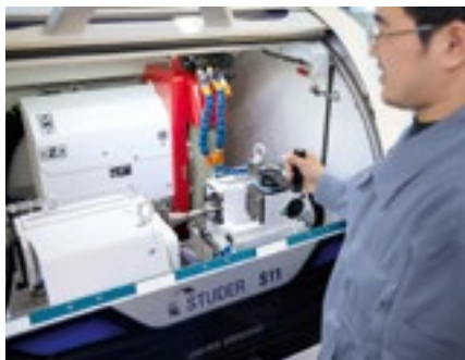
The center pressure on the rigid tailstock of the S11 can be set easily and sensitively
