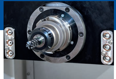
Coolant nozzles on grinding support for milling and drilling tools
