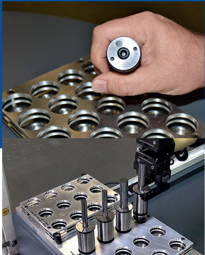
Customer project: Collet (type NK) with RFID system for automated regrinding with different tool diameters within a batch
