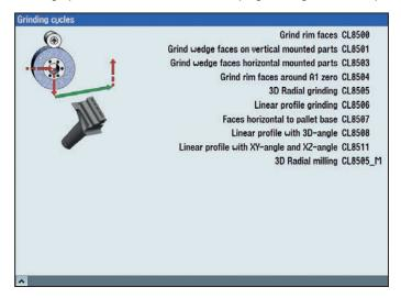
eces. In 5-axis machining, 3D grinding and auxiliary cycles can be programmed for milling and drilling operations.
