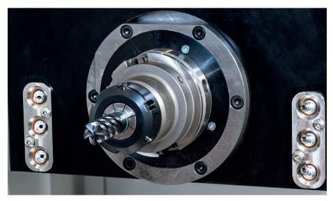
Nozzles are available on the grinding support for drilling and milling tools, and a coolant supply can be optionally provided through the spindle.
